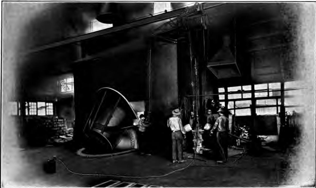
CASTING THE COPPER AROUND THE STEEL BILLET
